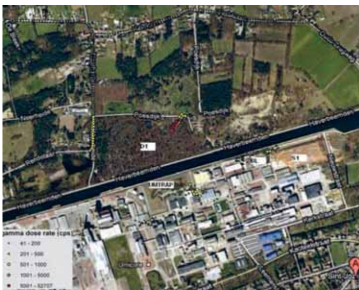
The Olen site – visible are the authorised disposal facilities “UMTRAP” and “Bankloop” (BL) as well as the former dumping sites D1 and S1. The dots correspond to external radiation measurements in counts per second. Dumping site D1 shows the highest rises.
